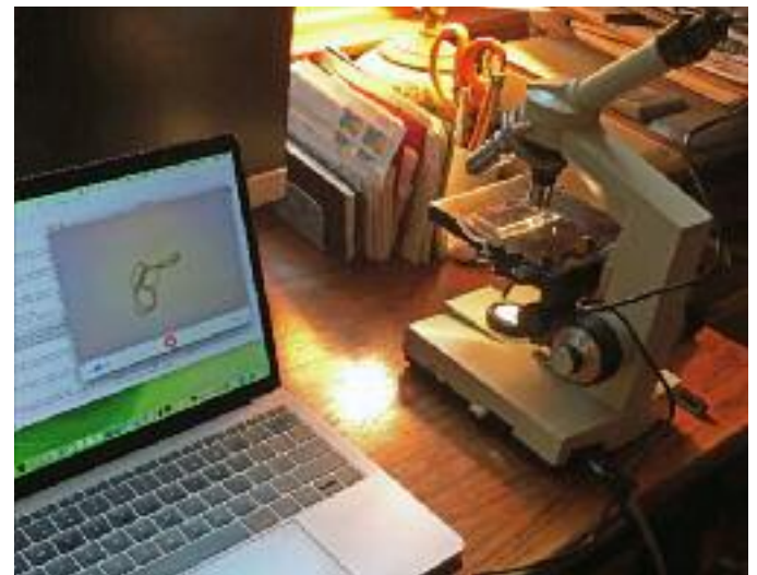
Microscope's computer interface displays any present cyanobacteria in ZAPPR's water sample.
