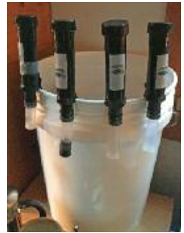
ZAPPRs concentrate each water sample's cyanobacteria at top of device.
